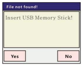
Solution →Insert USB drive to oven. If already connect USB drive to oven, wait for 5-10 sec. then click USB button on display. If Oven does not recognize, change USB drive.
